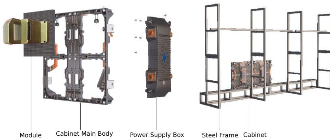
Exploded Diagram of Front Installation of Cabinet
